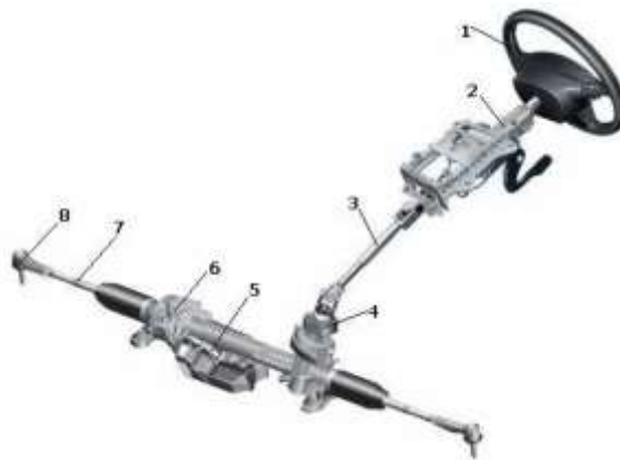
Figure 2. Rack and pinion steering structure:
